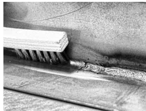
Cleaning a weld with a small scratch brush.
