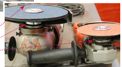
7" grinder (left) requires an adapting nut, where the 4-1/2" grinder (right) does not.
