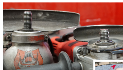
7" grinder (left) has a noticeably longer spindle than the 4-1/2" grinder (right).
