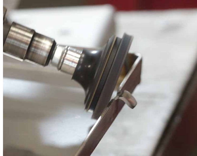
Edge chamfering a fabricated stainless steel component.
