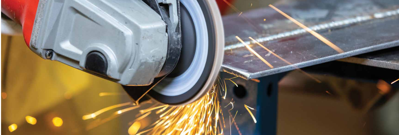
Tiger Paw grinding the edge of a torch-cut steel plate.
