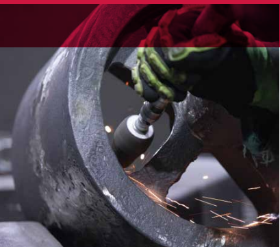
Using a cone to clean surface imperfections.
