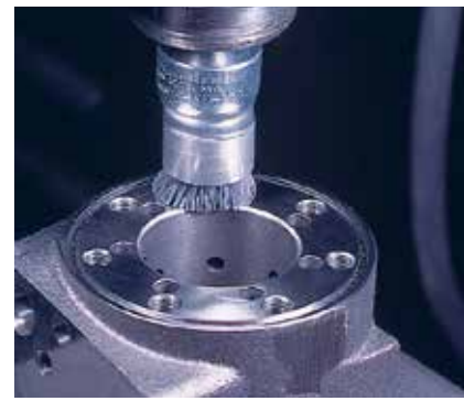
Blending tool marks on a hydraulic component.
