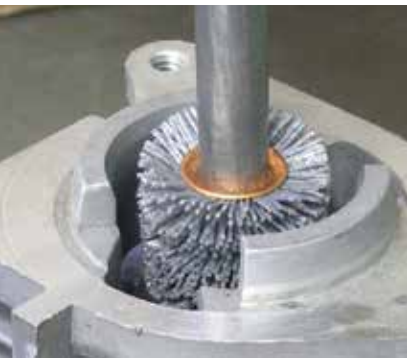
Deburring internal bores of a cylinder head.
