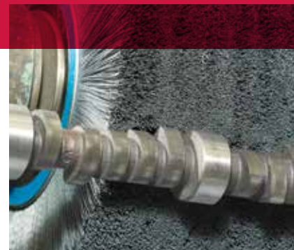
Deburring a camshaft with a Nylox wheel.
