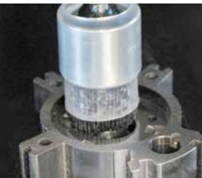
Deburring small features on a powdered metal part.
