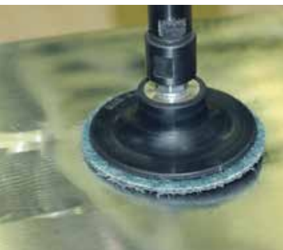
Finishing the surface for a stainless steel part for the food service industry.
