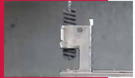
Deburring cross holes in a firearms component.
