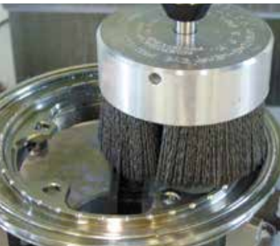
Removing burrs and breaking sharp edges on a transmission component.
