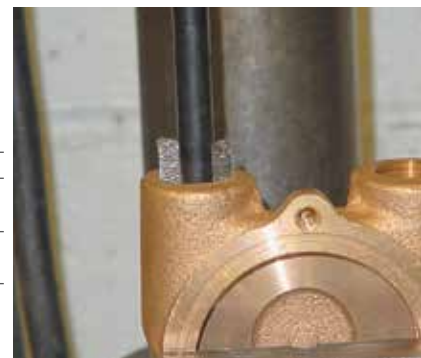
Deburring the threads of a tapped hole using a burr brush in a holder.
