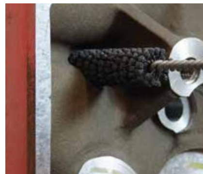
Cleaning burrs out of an automotive head port.
