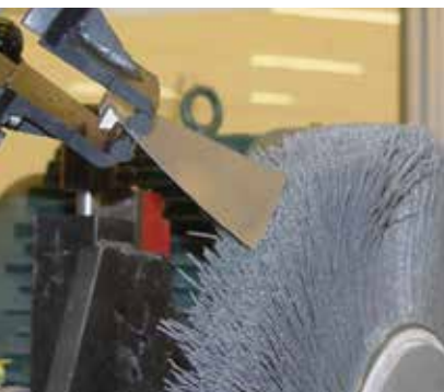
Deburring the tip of a turbine blade.
