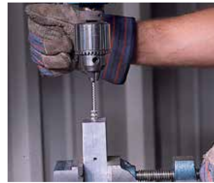
Crosshole deburring an aluminum manifold.
