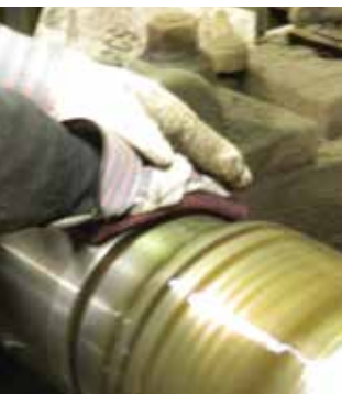
Finishing a rail axle journal with a non-woven hand pad.
