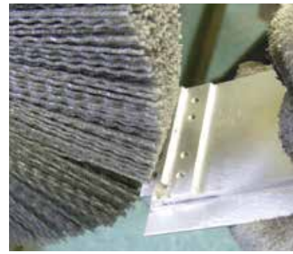
Removing burrs from an aluminum heat sink.
