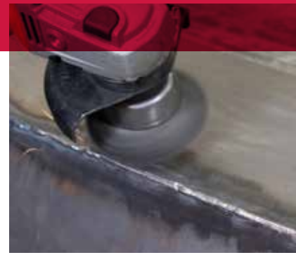
Knot wire cup brush removing heat discoloration.
