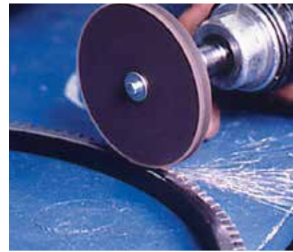
A unitized wheel deburring a ring gear.
