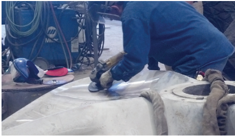
Tiger INOX grinding wheel blending a repair weld to the correct profile on a propeller blade. Tiger INOX offers a contaminant-free solution when working with stainless steel.
