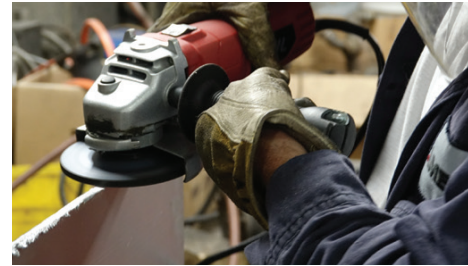
Tiger Aluminum grinding wheel prepping plates for welding. Tiger Aluminum offers a non-loading solution that will not contaminate the workpiece.
