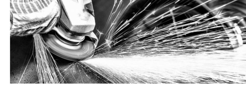
Applications: heavy stock removal, scale removal, weld removal, weld blending, edge beveling, grinding, notching, cutting, torch-cut edge softening Best On: steel, stainless steel, tooled steel, inconel, high nickel alloy, titanium, armored steel Tool speed and power: ceramic grains require high power tools that can mantain tool speed! Best result achieved with high power tools!
