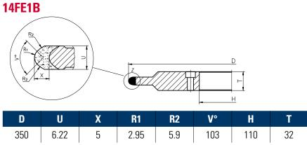
Grinding tools are produced according to the specification (depending on the dimensions of tools for rolling wires and grinding machine). Radius R1 can be made from 2,5mm to 20,5mm.
